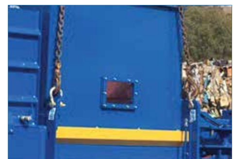
HOPPER VIEW WINDOW
