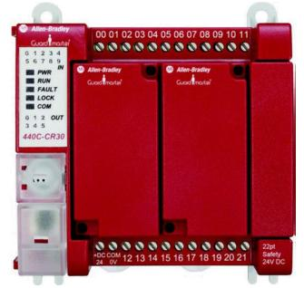
The CR30 safety relay can be configured to accept two single-wire safety inputs and to provide two single-wire safety outputs. This feature allows the CR30 safety relay to be an integral part of an extensive machine safeguarding system.
