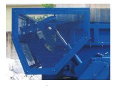
Force – Feed Ram An additional vertical force- feeding ram is available to pass the material onto the rotor from above in order to optimise performance.
