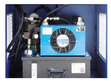
**Hydraulic Power Pack** Ram pressure and cycle time can be adjusted to suit different materials, oil cooler and dual- speed pump is also available to increase longevity and performance of the shredder.
