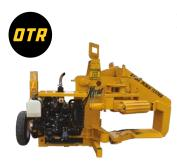
Designed to split OTR tyres into two halves down the center of the tread, the Punch Cutter is loaded onto a tyre with a telehandler and rotates around the outside of the tyre.
