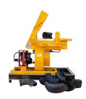
The Eagle TC Gator cuts the tyre clean and does not leave any additional chunks of rubber to remove after cutting each tyre.
