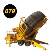
The Punch Cutter II is portable and designed to split OTR tyres into two halves, cutting through the center of the tread
