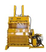
Designed to compress and bale whole car and pickup tyres, the Eagle 3060 reduces volume, fire hazards and makes it easier to transport tyres to processing stations.
